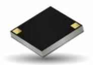
KYOCERA AVX custom thin film resistors are designed and tested for medical implantable and life sustaining applications. Methods and protocols include 100% automated electrical testing, life tests, MIL-883 visual inspection, design & process controls, reliability screening, and lot conformance testing.
