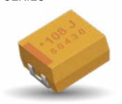
The T4J medical series are designed for applications other than implantable/life support utilizing KYOCERA AVX's **HRC4000** medical specification. These parts are designed to meet low leakage requirements and are processed using KYOCERA AVX's patented Q-Process which includes 125°C burn-in and statistical screening methods for high reliability assurance.
